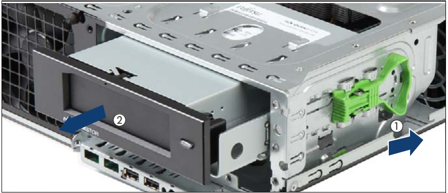
Figure 72: Removing the backup drive
